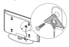
2 Mount a screw (not provided) to the wall or cabinet where your TV will be set. Leave the screw head protruding 1/4" (6.35 mm).
